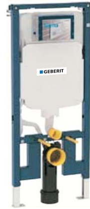
Duofix ** Cistern thickness: 8 cm Cistern height: 114 cm
